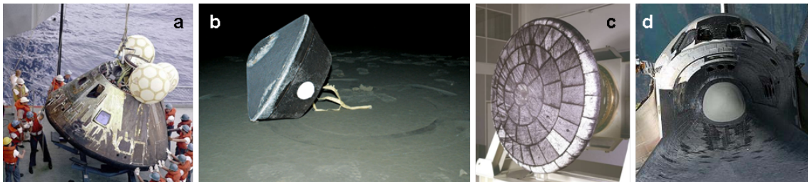
Figure 4: Re-entry vehicles: a) Apollo, b) Stardust, which performed hyperbolic re-entry in 2006 after having collected dust from the coma of comet Wild 2, c) European re-entry vehicle ARD (Atmospheric Re-entry Demonstrator), which completed re-entry flight from a sub-orbital mission after launch with Ariane 5, d) Space Shuttle, which operated on 135 missions from 1981 to 2011.
