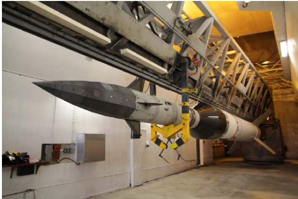
Figure 8: Payload of the SHEFEX II re-entry vehicle on the launcher on June 22nd 2012.
