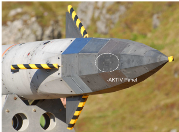
Transpiration-cooled experiment AKTiV on SHEFEX II.
